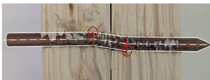
Failure mode: double plastic hinges - EC5: F FIR - SHEAR 2
